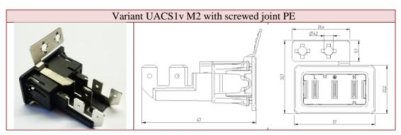
Variant M2 with two 6.3 mm blade connectors according to DIN EN 61210 on the power carrying contacts and a screwed joint protective earth with one blade connector
