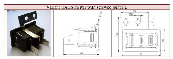
Variant M1 with one 6.3 mm blade connector according to DIN EN 61210 on the power carrying contacts and a screwed joint protective earth without blade connector
