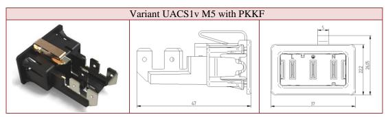
Variant M5 with two 6.3 mm blade connectors according to DIN EN 61210 on the power carrying contacts and a special innovative metal spring connection called "PKKF = Powerkontaktklemmfeder" on protective earth with one blade connector
