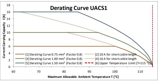
Derating curves<sup>5</sup> UACS1 according to DIN EN 60512-5-2, Variant with 6.3 mm connectors
