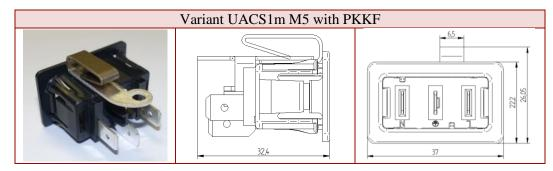
Variant M5 with one 6.3 mm blade connector according to DIN EN 61210 on the power carrying contacts and a special innovative metal spring connection called "PKKF = Powerkontaktklemmfeder" on protective earth with one blade connector
