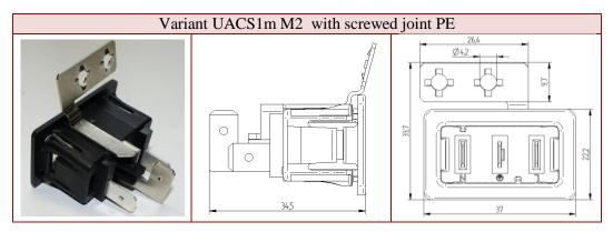
Variant M2 with one 6.3 mm blade connector according to DIN EN 61210 on the power carrying contacts and a screwed joint protective earth with one blade connector
